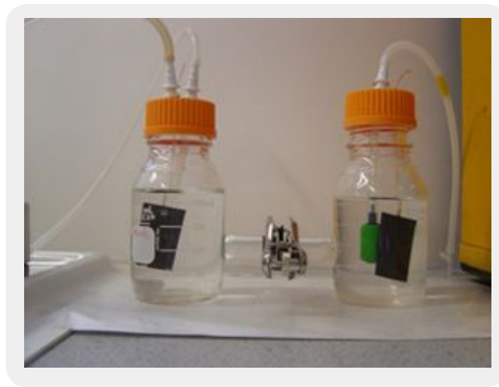
Figure 2: A simple two-chamber system microbial fuel cell [29]
